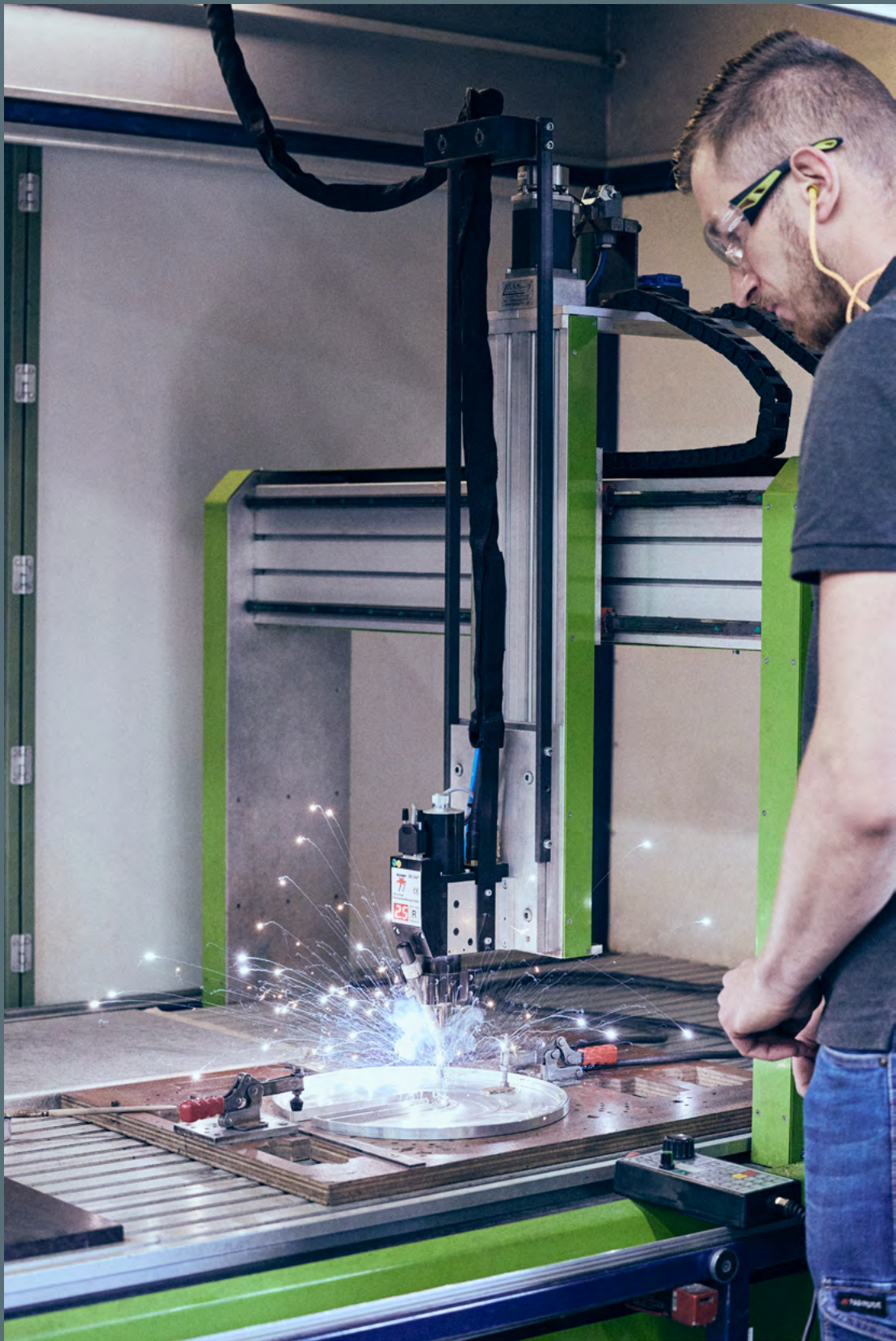
Spot welding: The image shows three bolts being welded onto the Naxos reflector . This enables the LED boards to be securely screwed in place and ensures that they can be easily replaced.
