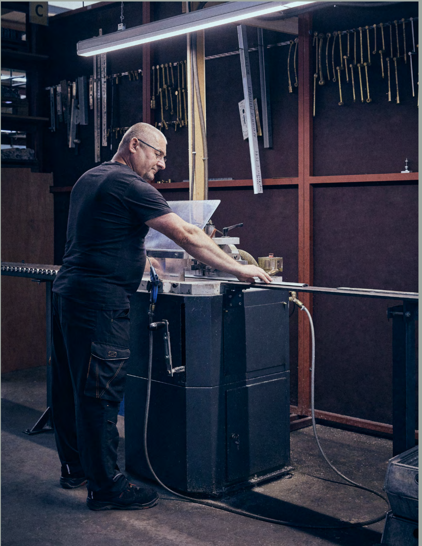
Cutting aluminum profiles. The image shows the profile of the Epsilon pendant light .
